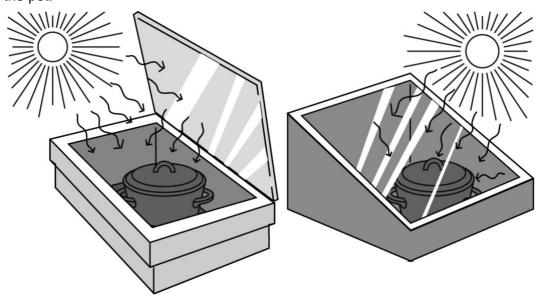
The top of the box is covered with glass or clear material that can allow sunlight to enter the box and trap heat. The inside of the box should be black, ideally, to absorb heat. An adjustable reflector can be attached to the top of the box to direct more heat and light onto the pot
