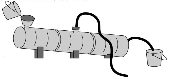
This picture shows a system made from 3 drums. The manure goes in at the top end, the gas rises and is taken away using the pipe in the middle, and the slurry is taken from the other end and used to enrich the soil and strengthen the Nature Cycle. The drums could be on a natural slope instead of a stand. The designs are endless!
