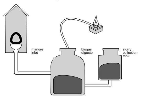
Organic matter (like manure and fresh plant scraps) is put into a 'digester'. Water is added. The digester works like a stomach to digest food. There are many different ways to put this material in the digester. It can be a part of the regular sewage system or there can be a door or opening to add the organic matter (then close it again so the gas does not escape). Organic matter should be added often so that gases are always being made. Water will need to be added too.
