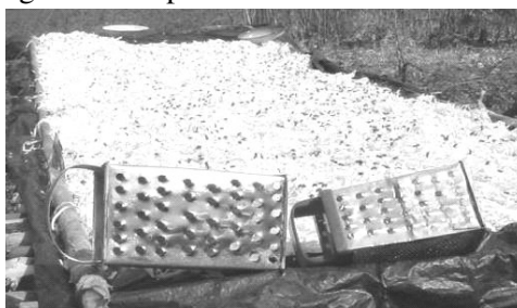
The grater on the left is made by a local tinsmith, the right one was imported from South Africa. After processing of about 1.000 kg of fresh cassava it was worn out.
